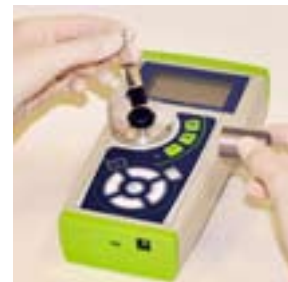
Measuring micronutrient content with the iCheck™ T3 spectrofluorophotometer (lower image); the complete kit in its convenient carrying case (upper image)
